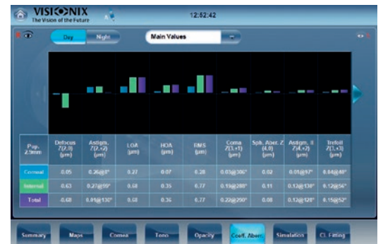
Analysis of aberrations with Zernike coefficients
