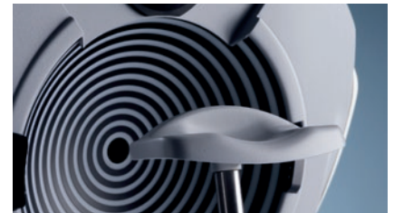
Placido disk - Measurement of corneal curvature radius
